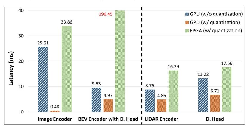
**Observation 3**: The quantized BEVDet on the GPU is superior for PDP performance. Lower PDP achieved on FPGA for LiDAR encoder and detection head.
