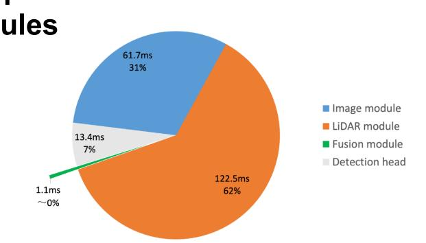
Main bottlenecks are image, LiDAR module and Detection Head
