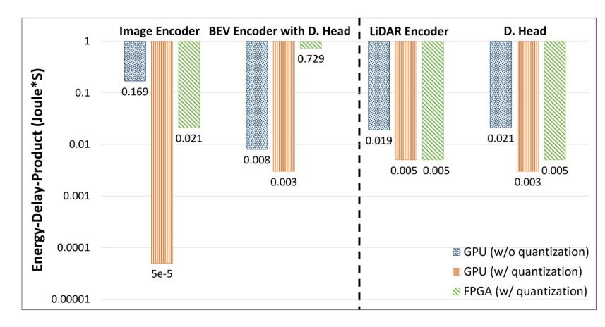
**Observation 4**: The quantized image encoder and BEV encoder with a detection head perform better on the GPU. The quantized LiDAR encoder and its detection head are equally efficient on both the GPU and FPGA.
